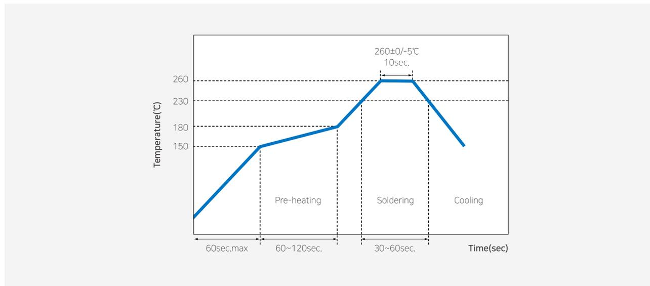
[Reflow Soldering Conditions]
